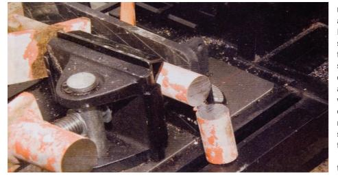
revving motor turned the blade quitely and it went through the steel in seconds. I put hardly any pressure on the handle so it is certainly the blade that is doing the work. The cut was very clean and square so it is an ideal machine for cutting steel plumbing pipe, which needs a thread cutting, and it will also work very well on a threaded bar or studding as we call it in my part of the world. In all the metal cutting exercises the tiny chips of steel were collected in the removable tray.
