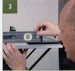
Check and adjust the table extensions until they are all aligned and level
