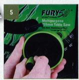
Even with easy blade adjustment always, once adjusted, make a cut on scrap timber to check it first
