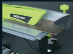
SCIE S/ TABLE: PLAQUE D'ACIER 3MM
