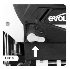
This jigsaw has a 4 position switch (0-3) located on the Left Hand side of the machine just behind the blade. Only operate this switch when the machine is switched 'Off' and the blade is stationary.
