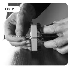
**Note:** The Battery Pack must be disconnected from the machine when installing or removing the blade.
