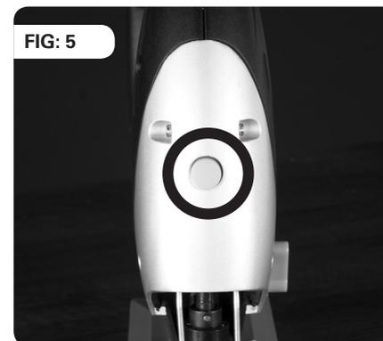
Only switch the Laser Guide on when you are about to make a straight cut, and switch it off when the cut has been completed. The switch is located on the front of the machine. Press the button once to switch the Laser Guide 'On'. Press once more to switch the Laser Guide 'Off'. **(Fig. 5)**
