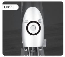
Only switch the Laser Guide on when you are about to make a straight cut, and switch it off when the cut has been completed. The switch is located on the front of the machine. Press the button once to switch the Laser Guide 'On'. Press once more to switch the Laser Guide 'Off'. (Fig. 5)
