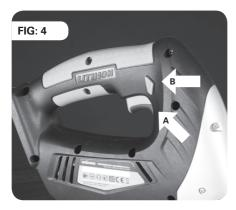
The Trigger Switch can only be operated once the safety lock has been disengaged.
