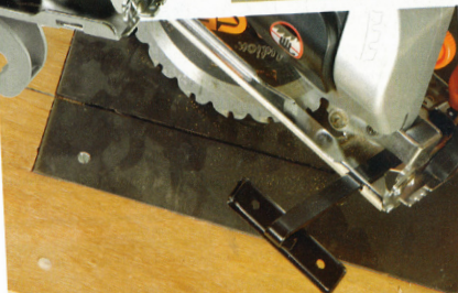
A This steel plate is 4mm thick and the ply is 19mm. The saw didn't flinch!
