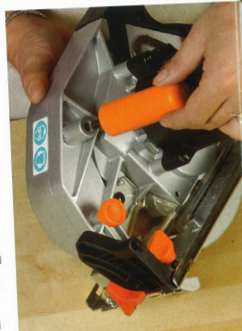
A The front handle can be moved back to a middle position if necessary
